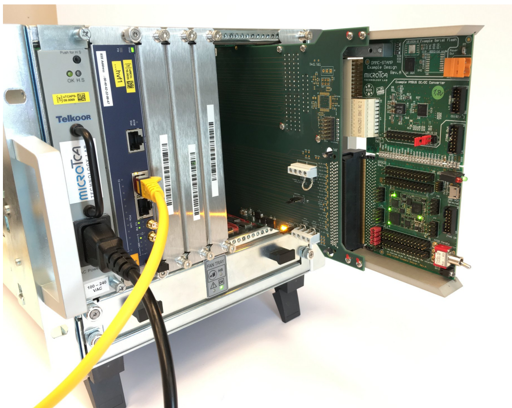
Figure 4: DMMC-STAMP-BoB installed in a MicroTCA system
